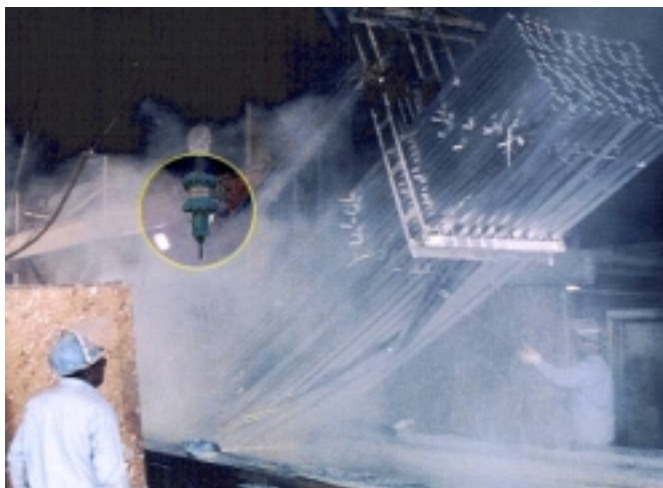
Pneumatic Vibrahoist removing excess zinc after hot dip galvanizing
