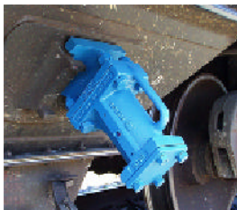
Left: HCP - Hopper Car Portable Vibrator
