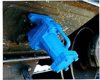
NAVCO HCP Vibrator ensures material flow from rail cars.
