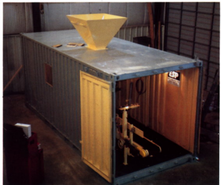
Typical sea/land container supplied by customer, modified by E.S.P. to house a complete bagging operation for handling hazardous waste products.
