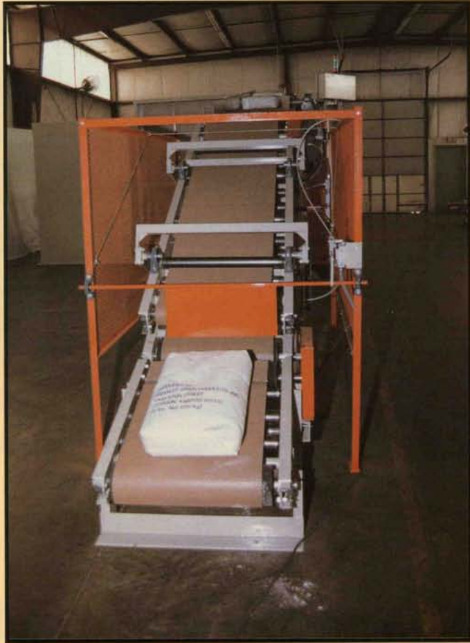
View of bag entering flattening conveyor system shown with standard safety cages
