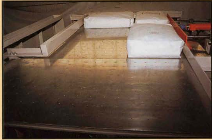
Operator view of fixed and moveable air flotation tables
