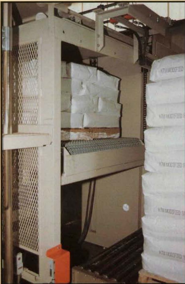
Moveable conveyor with pallet being filled.
