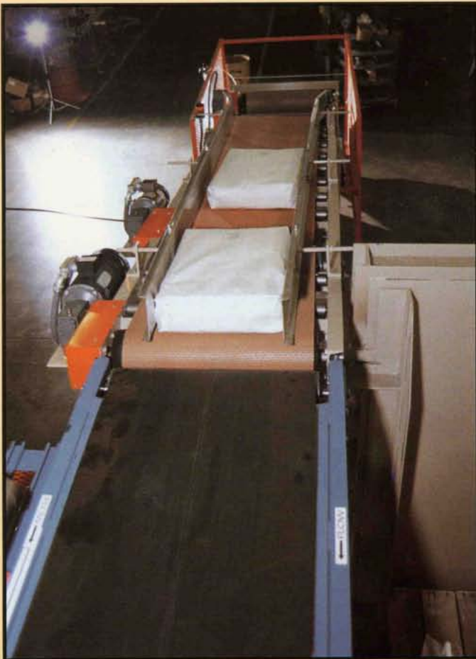
Accumulation conveyors bringing flattened bags onto optional check weigh system
