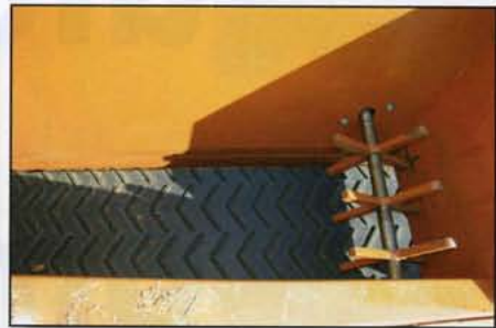
Cleated, incline belt and agitator
