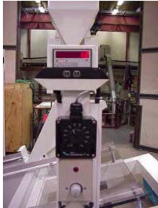
Controls for adjusting the vibratory feed and belt speed are conveniently located for the operator.
