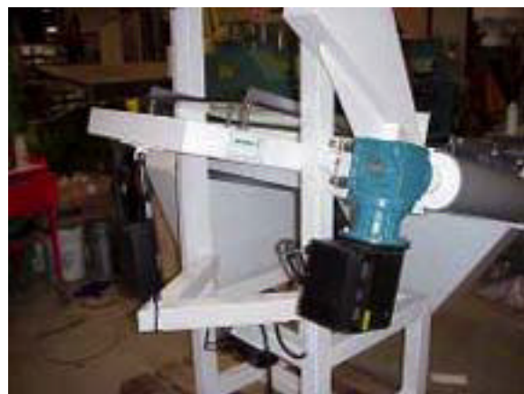
Electronically variable speed belt drive enables the operator to fine tune the belt speed to achieve the best separation.
