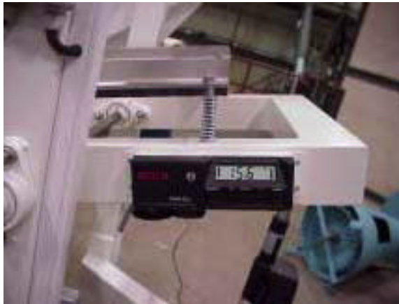
Digital control unit for adjusting the belt side inclination. This makes it easy for the operator to duplicate seed conditioning lots and to control the separation.
