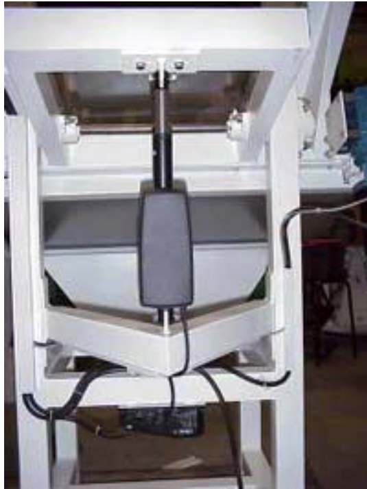
Electrical control for changing the side inclination angle of the belt. Note the pivot point for adjusting the incline.
